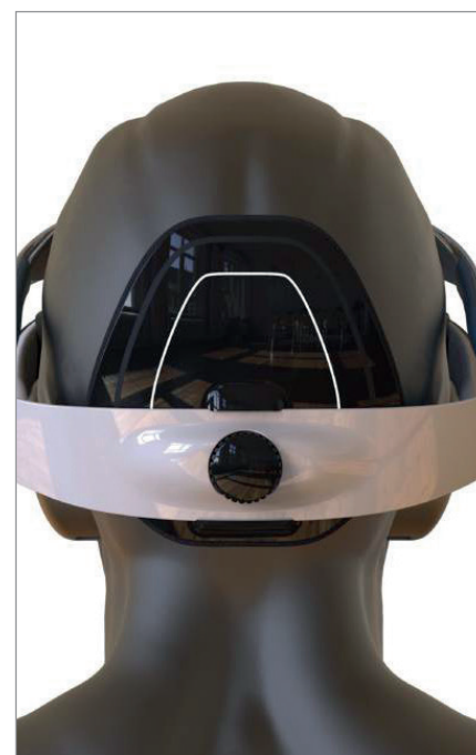
Figure 1: The nGoggle: a portable system for objective assessment of visual field deficits
