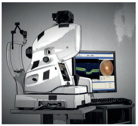
Figure 1. An OCT instrument that requires a PC running Windows XP for image acquisition.
