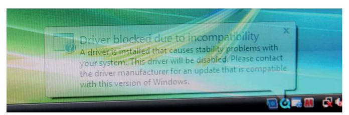
Figure 2. Later versions of Windows can break the functionality of the device drivers you need for your instrument to work - meaning that you cannot upgrade.
