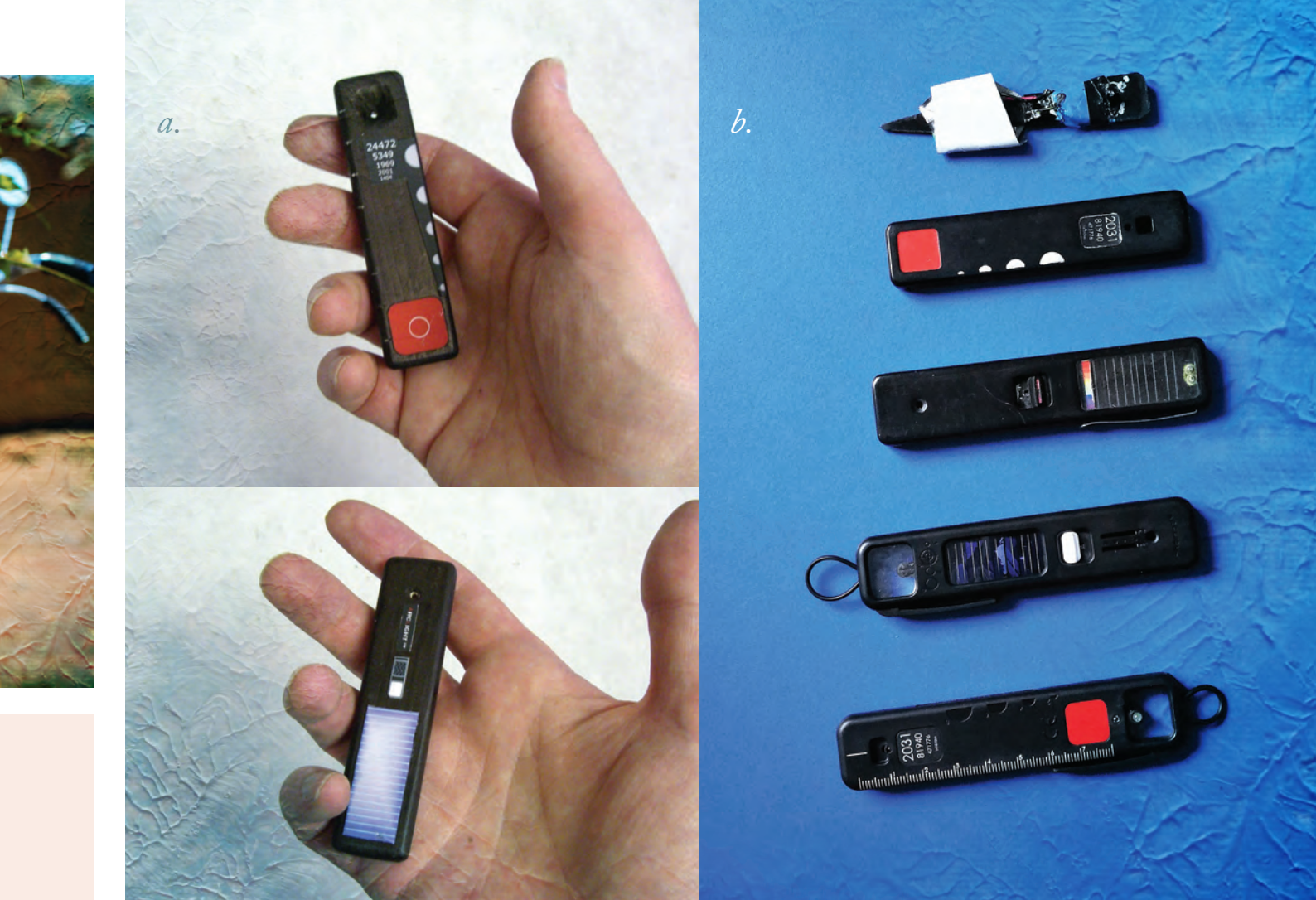
Figure 2. a. Wooden mock-up version of the Arclight. b. Prototypes of the device with additional features. The prototype at the top is the original prototype created from a popsicle stick.
