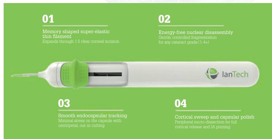
Figure 1. The pen actuator allows the nitinol loop to be inserted through a clear corneal incision and then expanded to encompass the lens. Constriction of the loop results in atraumatic, energy-free bisection of the lens, independent of cataract grade and without stressing the capsule. Loop movements have a capsular sweeping and polishing effect.
