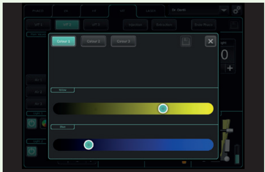
Figure 3. Adjustable colors on the Oertli OS4®'s Goodlight® LED. Users can set any ratio of their choosing and save up to three different ratios in the device's memory.
